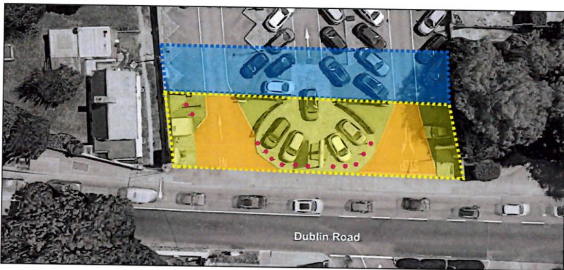
Figure 7.0 Aerial view of site access and egress illustrating the anticipated area to be permanently (yellow) and temporarily (blue) acquired by the NTA. Note the bollards to be removed and replaced along the boundaries (pink dots) and the reduction in width afforded to the access and egress which have been critical in providing a safe access to site due to optimal visibility (orange).
